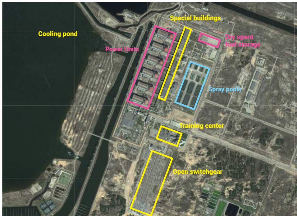
Some facilities and structures at the Zaporizhzhia NPP site. Author's diagram on Google Earth satellite image.
